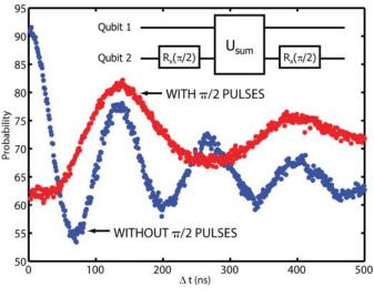
protocol with the extra  $\pi/2$  pulses. Both measurements were carried out using the same microwave power for the sum frequency. The used microwave frequencies were 10.878 GHz for the sum-frequency transition and 6.889 GHz for qubit 2. The microwave sources were phase-locked together with the chopping pulse. The oscillation period is doubled in the case of the protocol, as expected.
